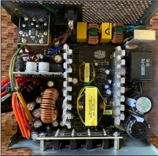
The main materials used are in the robust metal housing (steel alloy), the transformer and inductors (e.g. copper and ferrites), the passive cooling elements (aluminium), the fan (plastic) and the printed circuit boards (glass, epoxy, plastics, solder).
