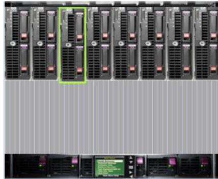
Figure 16: Illustration of a blade system
